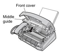
Clean the document feeder rollers with a cloth moistened with isopropyl rubbing alcohol, and let all parts dry thoroughly.
